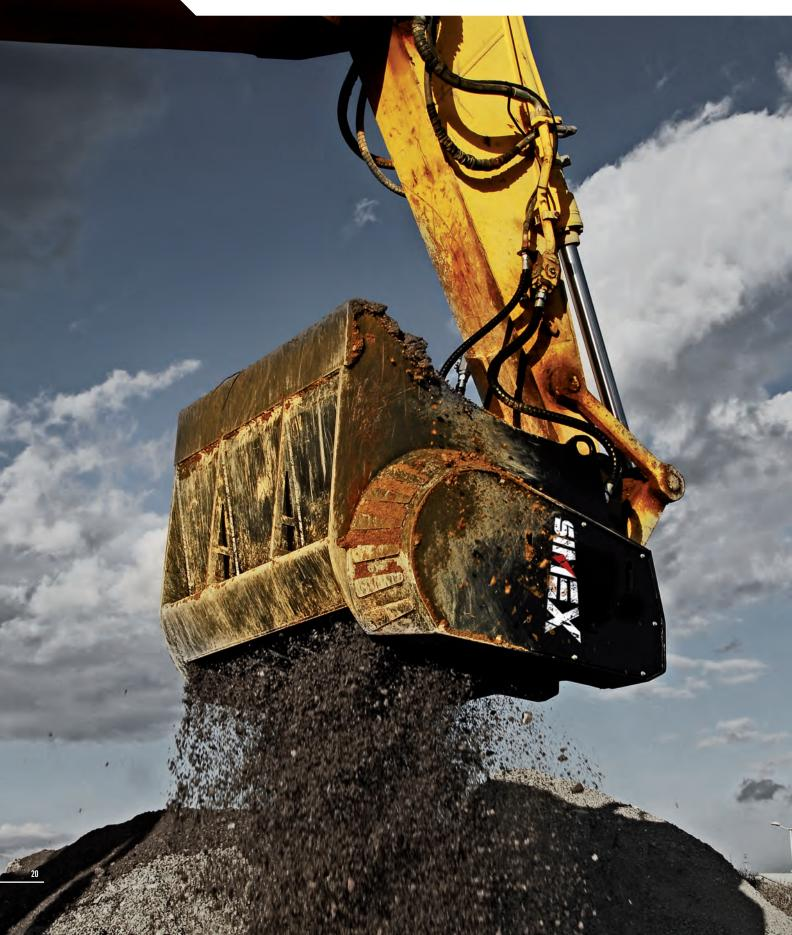
■ Designed for **separating different-sized materials** on the work site.
